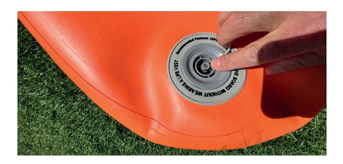
4) Insert the end of the tube into the valve and turn it  $\frac{1}{4}$  of a turn clockwise to hook it to the valve
